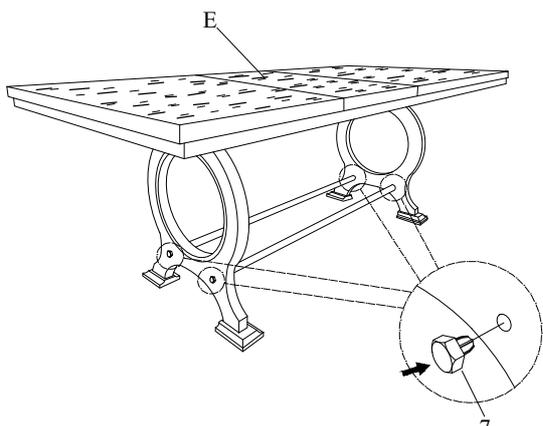
\*\*\* Notes : 1. Do not fully tighten the nut or bolt until all nuts and bolts are attached.
